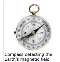
Compass detecting the Earth's magnetic field
