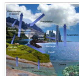
Schematic of the hydrologic cycle components in present-day setting [see Annex 3, p. 15]
